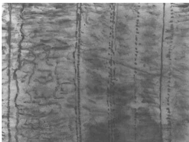
Fig.3 Translational deformation mode in copper visualized by the NLC. 60* magnification, t = 20^{\circ}\text{C} .
